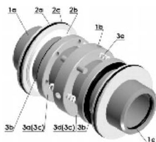
A CAD model of a mechanical double seal
