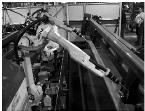
A set of six-axis robots used for welding.
